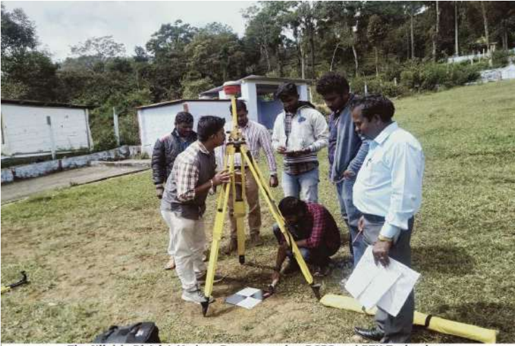
The Nilgiris District-Modern Resurvey using DGPS and RTK Technology
