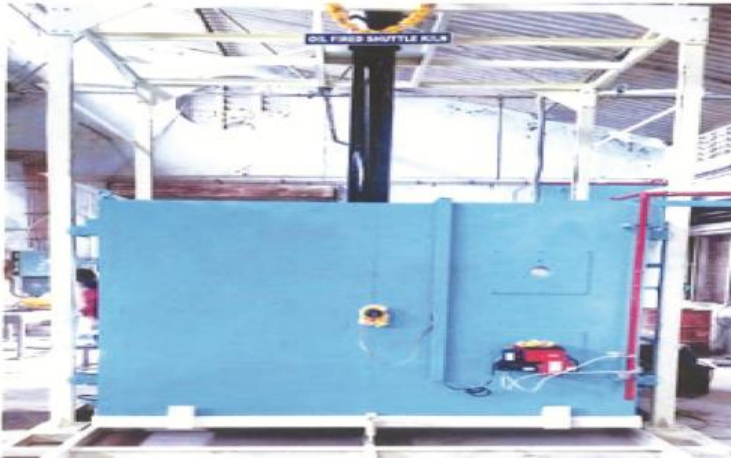
Oil fired shuttle kiln at Art pottery unit, Virudhachalam
