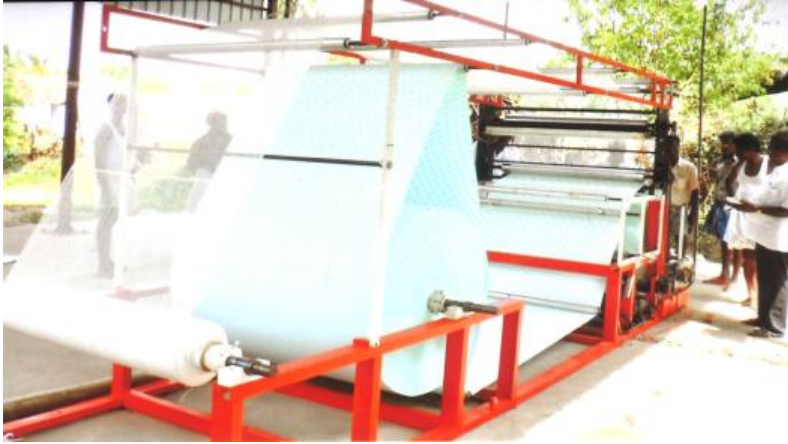
Cloth lined cover manufacturing machine at HMP unit, Govanur
