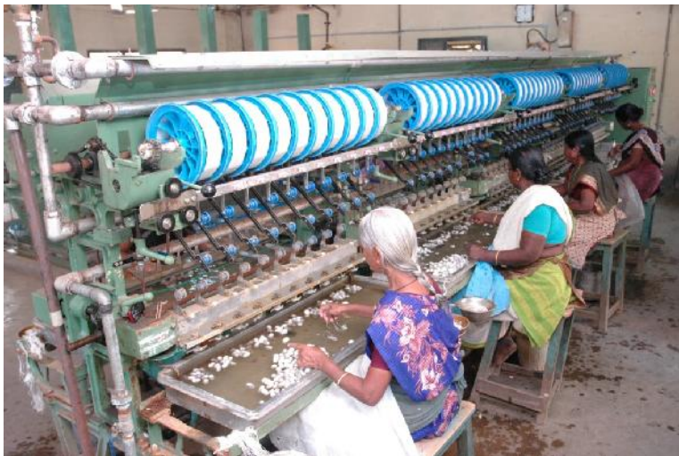
Newly installed Multi-End Reeling Unit at Salem
