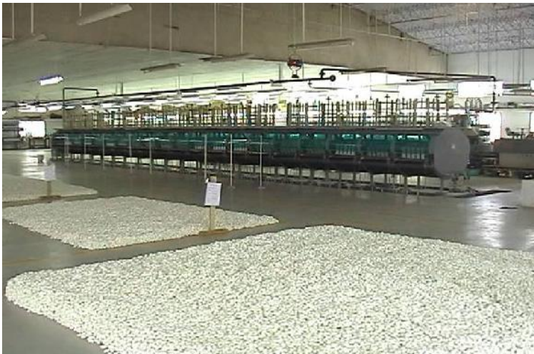
Automatic Reeling Unit at Avinashi
