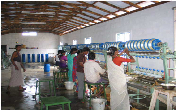
Multi-End Reeling Unit at Dharmapuri
