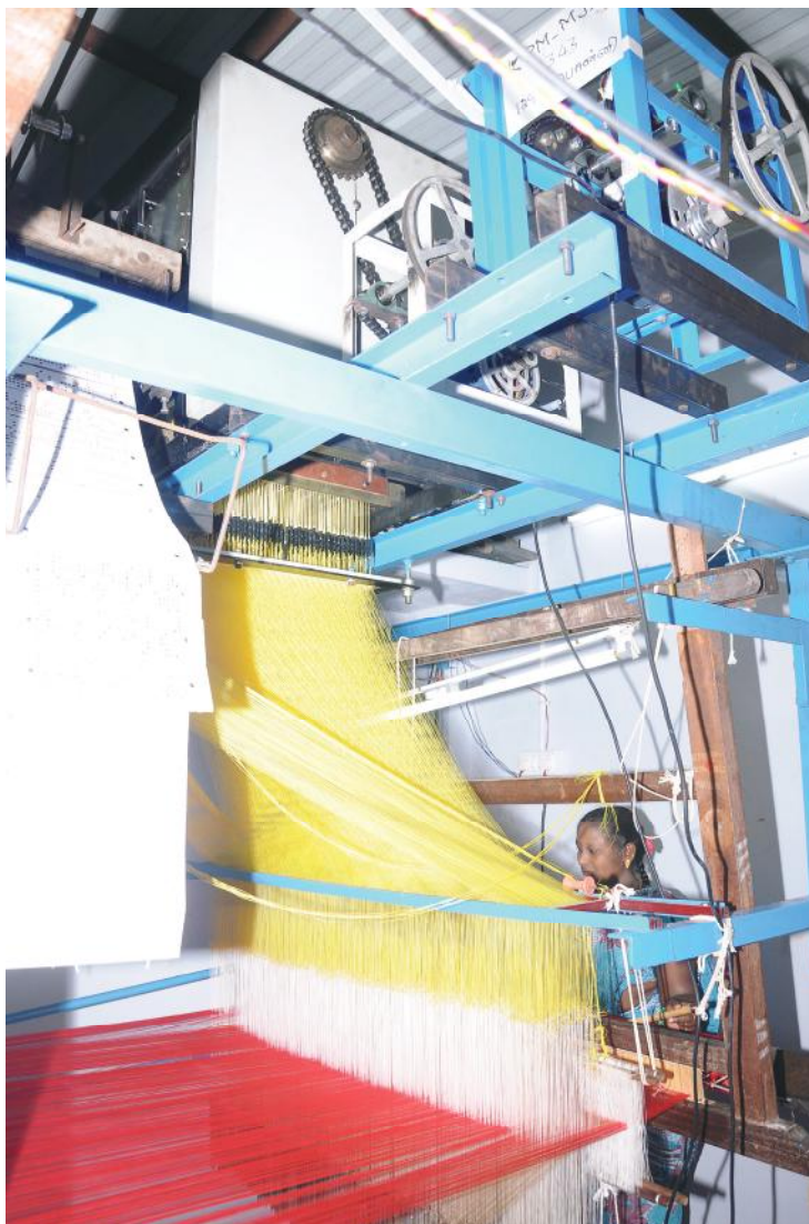
Weaver weaving in Handloom fitted with Motorized Jacquard Lifting Machine
