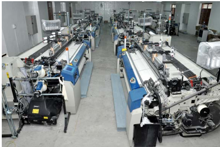
New Automatic Shuttleless Powerloom (Airjet Looms) Installed at Tamilnadu Textile Corporation Ltd.,Coimbatore
